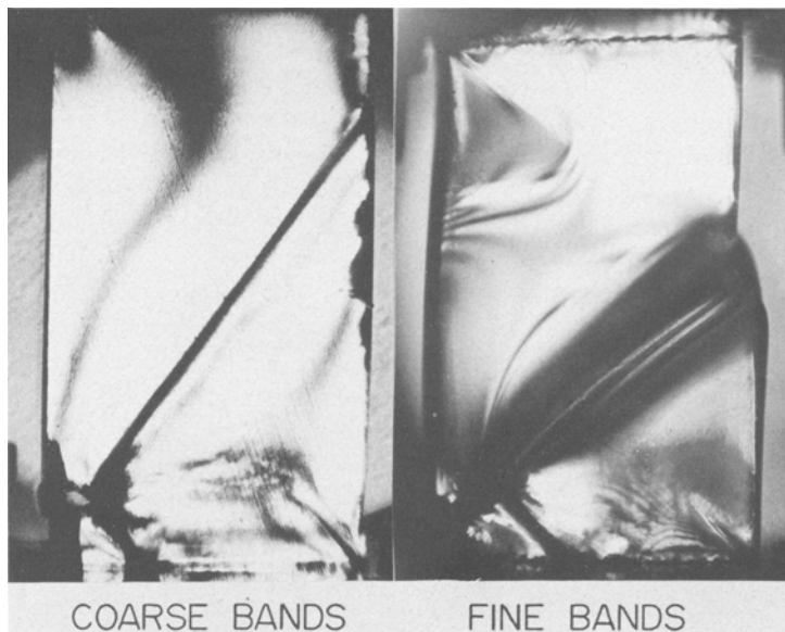
Figure 18 Difference in ductility of coarse and fine slip bands.
